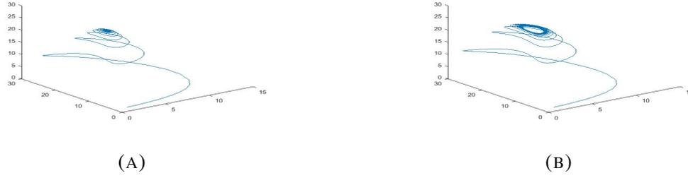
FIGURE 6. Hopf Bifurcation. (a) The system is stable when  $U^* = 0.3$  and  $t_1 \leq 0.8$ ; (b) The system is unstable when  $U^* = 0.3$  and  $t_1 = 0.9$
