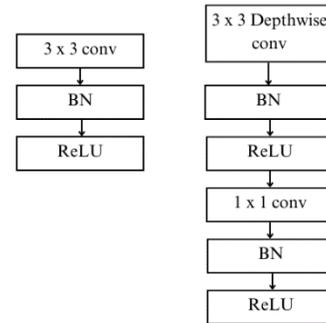
Figure 2. Batch Normalization and Rectified Linear Unit after each convolutional layer
