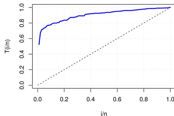
FIGURE 3. TTT Plot for Fatigue Life Analysis of 6061-T6 Aluminum Coupons data set
