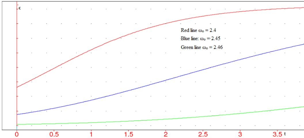
Figure 4. Curves exhibiting the dependence of the strain-time relationship on the natural frequency  $\omega_o$ .
