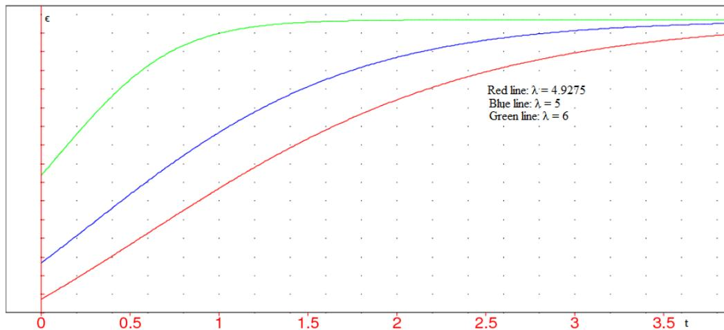
**Figure 3.** Curves showing the effects of the damping coefficient  $\lambda$ .
