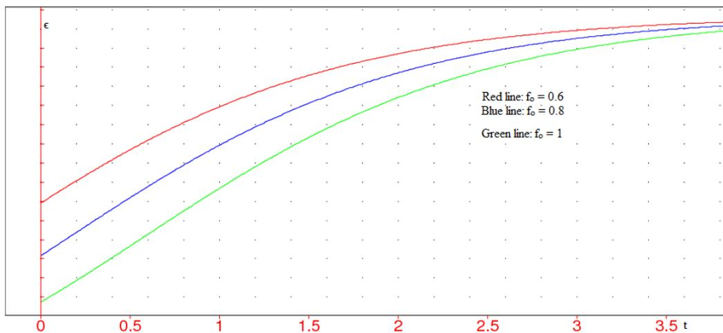
Figure 5. Curves illustrating the effects of the parameter  $f_o$  action on the strain-time relationship.
