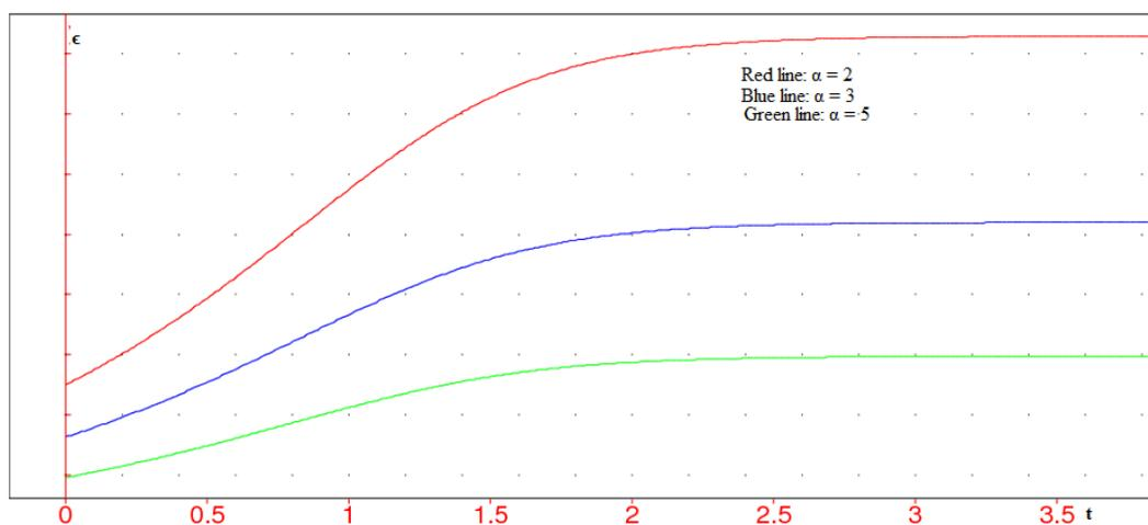
Figure 2. Strain-time curves showing the effects of the material coefficient  $\alpha$ .
